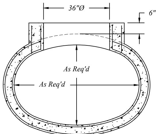
Pipe Manufactured To ASTM C-507
